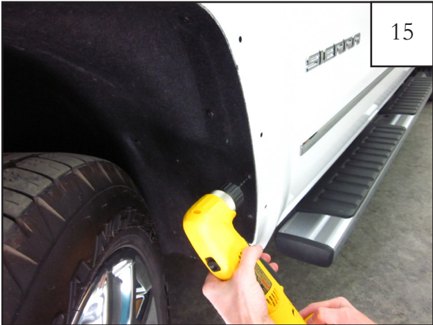
15 Remove the flare. Using a 3/32" drill bit, drill a pilot hole through the factory wheel well liner and sheet metal at location marked in previous step.
