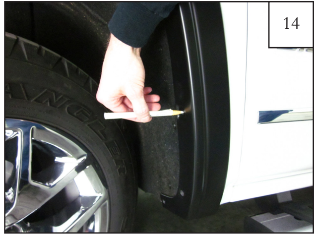
14 Using a grease pencil or marker, mark one hole location for drilling using the upper rear hole location in the flare as a guide. Note: This step not needed for models with factory installed mudflaps.
