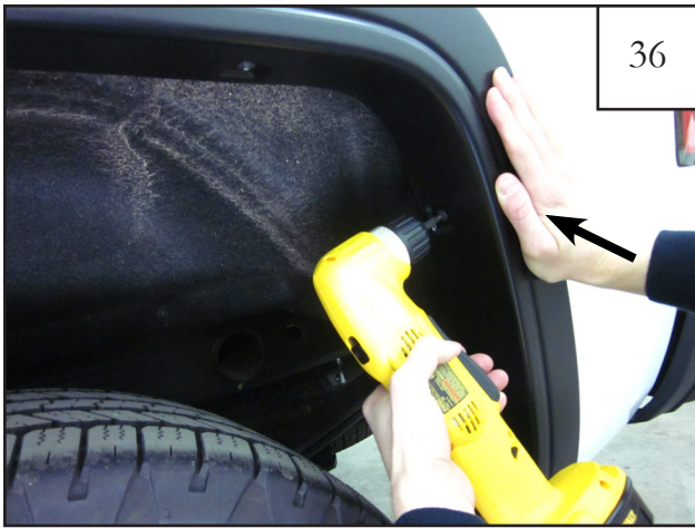
36 Install self-tapping screws (SW1-0066) into pilot holes drilled in step 31 (3 places). Press flare firmly towards the vehicle while fully tightening.
