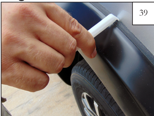
39 Using supplied Edge Trim Tool (ET1-0002), seat edge trim against vehicle by hooking curved end under edge trim at one end of flare. Next, slide around outer edge of flare to the other end.
