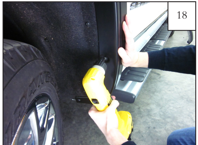
18 Install self-tapping screw (SW1-0066) into pilot hole drilled in step 13. Press flare towards vehicle while fully tightening. Note: This step not needed for models with factory installed mudflaps.
