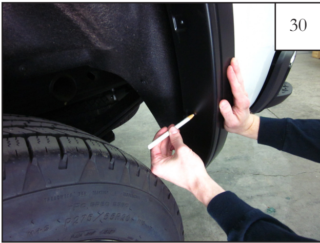
Using a grease pencil or marker, hold flare in place on vehicle and mark hole locations for drilling (3 places).
