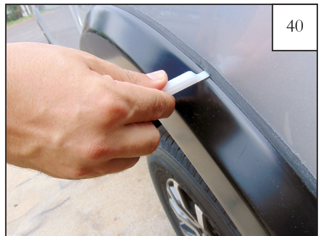
40 Using flat end of supplied Edge Trim Tool (ET1-0002), seat edge trim against flare by inserting straight end between edge trim and flare at one end. Next, slide around entire edge to the other end.
