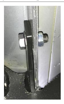
**Step. 6:** After finial positioning, completely tighten all (x6)  $\frac{1}{4}$ "-20 x  $\frac{3}{4}$ " in the pinch weld attachment.
