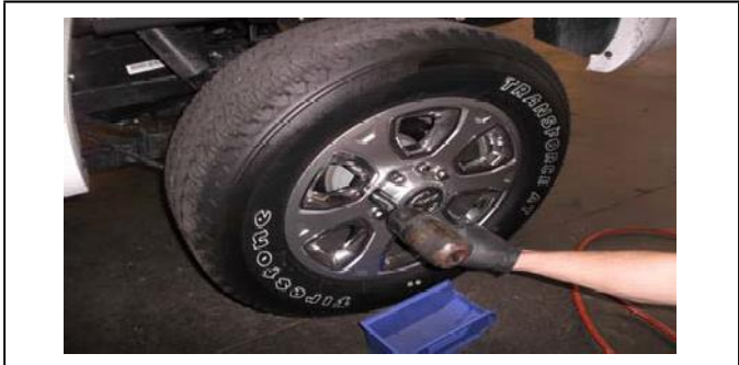
30. Reinstall the rear wheels.
