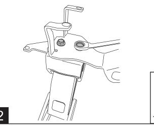
Drop threaded plate into slot in frame. Slot is located on both sides of the frame. The outer slot is preferred but may not be accessible with aftermarket bumpers or racks.
