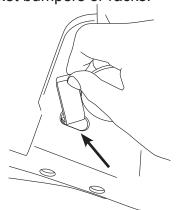
Set assembly into position and replace hardware from step 1. A M10 bolt and washers are supplied if bolt is not present. Do not tighten.
