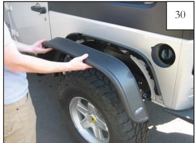
Place the outer flare over the inner pieces and push until snug against the vehicle surface. Make sure splash shield is tucked behind flare.
