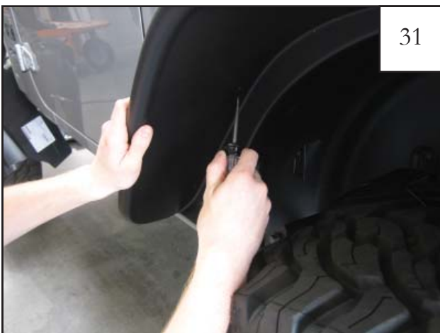
Use a scratch awl (or another pointed tool) to line up the speed clips with the outer flare holes (6 locations). If needed, use a flashlight to better locate the speed clips.
