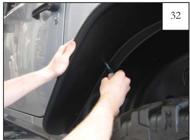
Hold flare in place on fender and start a pan head screw into each hole location and through the speed clip on inner structure (6 locations). Do not tighten.
