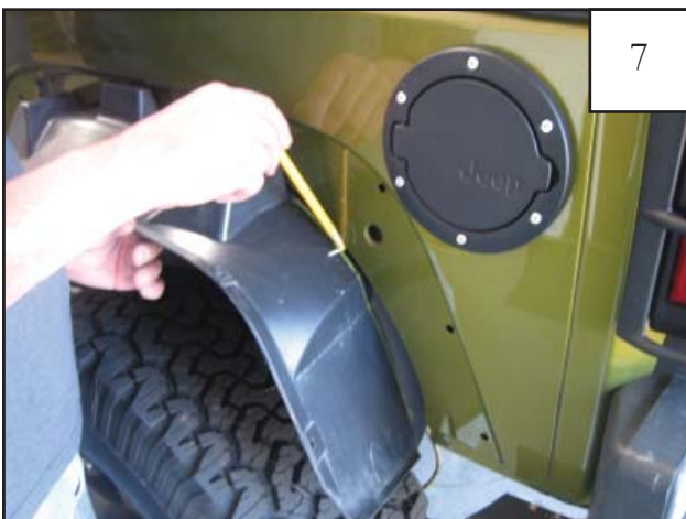
Using sheet metal as a guide, mark the splash shield with a grease pencil in preparation for trimming. The splash shield should be flush with the sheet metal after being trimmed. NOTE: If trimmed too little, flare won't fit; if trimmed to much, shield won't stay behind flare.
