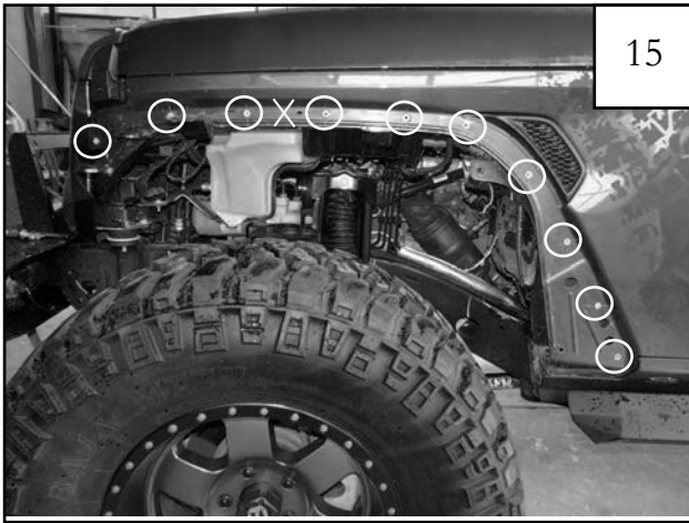
Ten rivnuts installed. NOTE: The "X" above indicates a hole that is not used.
