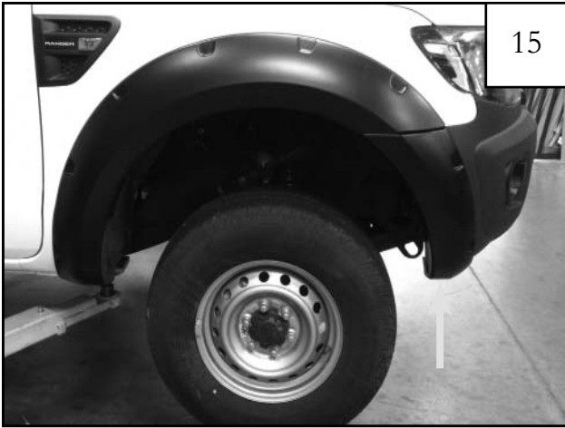
Using a 10mm socket wrench, install the factory bolt that was removed in step 8 under the front bumper area of wheel well.
