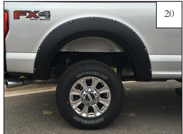
20 Completed rear flare installation.
