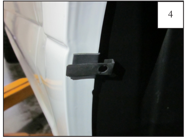
Install a Clip (CL1-0009) over the Tab (MT1-0034) placed in Step 3.
