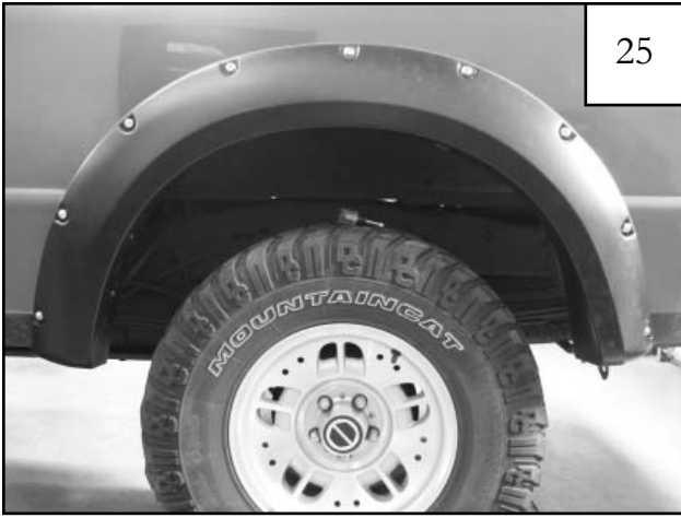
Completed rear flare installation.
