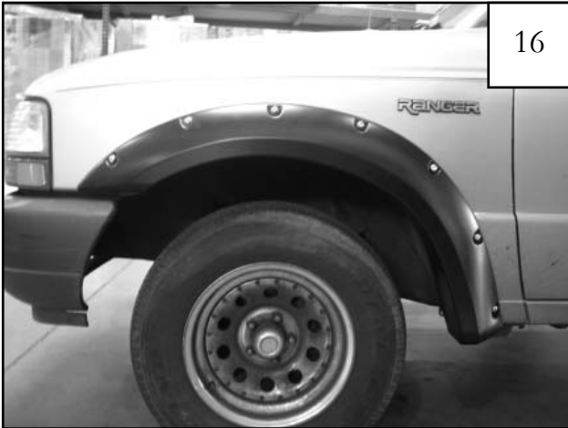
Completed front flare installation.
