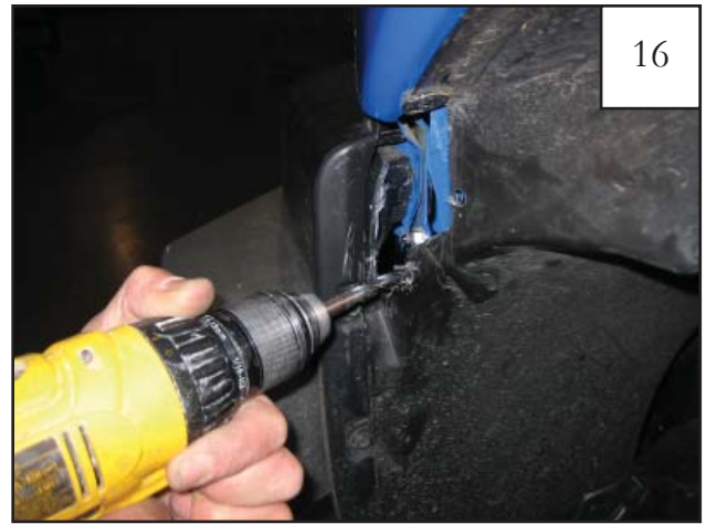
16 Remove Front Inner Piece, and drill two 5/16" holes on marks made in previous Step (2 places).
