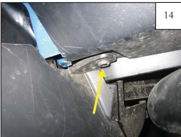
Remove third mud flap bolt, and remove mud flap.
