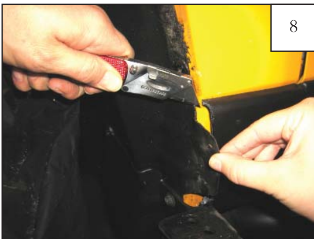
Using a utility knife, cut splash guard flush with edge of sheet metal also.
