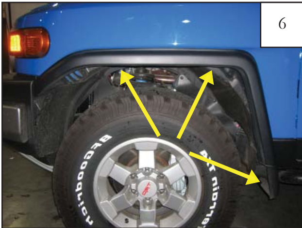
Remove three plastic fasteners using a flat head screw driver or pry tool.
