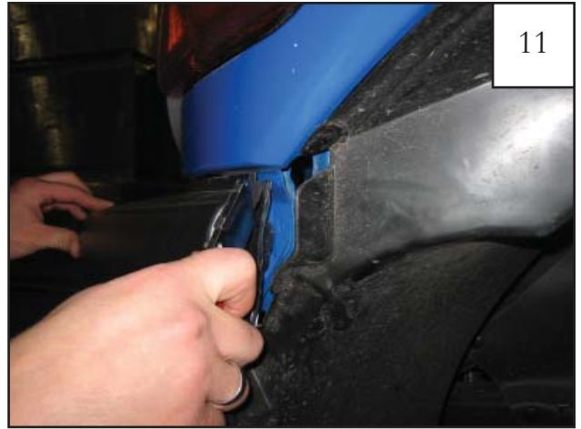
Trim remaining plastic flush with bumper.
