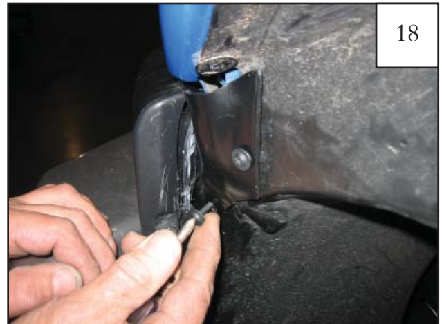
18 Position Inner Front Piece on vehicle, aligning holes in part with holes in Clips installed in previous Step. Install supplied Screws (SW1-0056).
