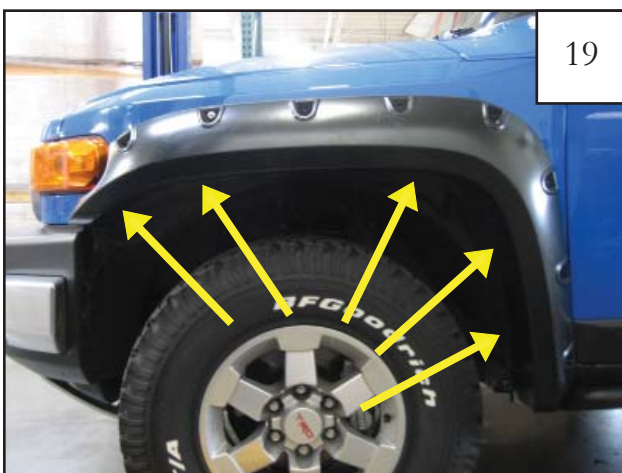
19 Position Flare on fender. Install five supplied Screws (SW1-0036). Do not tighten. NOTE: It is helpful to install one of the top bolts first.
