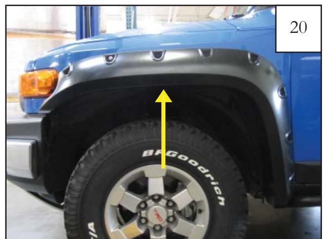
20 Install one supplied Fastener (RV1-P003) in top hole. Check that Edge Trim (GP1-0001) is seated correctly, then tighten all Screws (SW1-0036) installed in previous Step..
