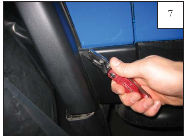
Using a utility knife, cut along seam connecting factory flare to rocker. Cut down to mud flap area.
