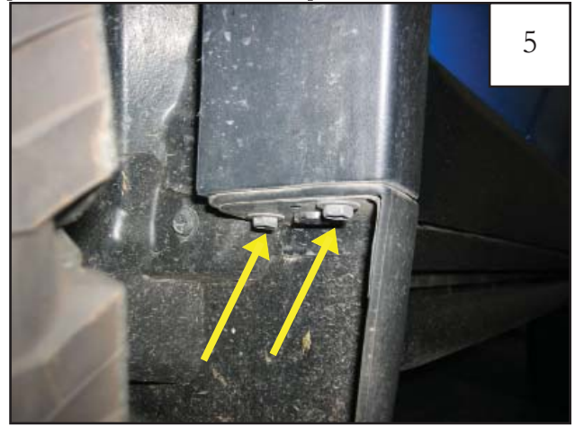
Remove two bolts connecting factory flare to rocker as shown (one plastic fastener removed in Step 4 is located here as well).
