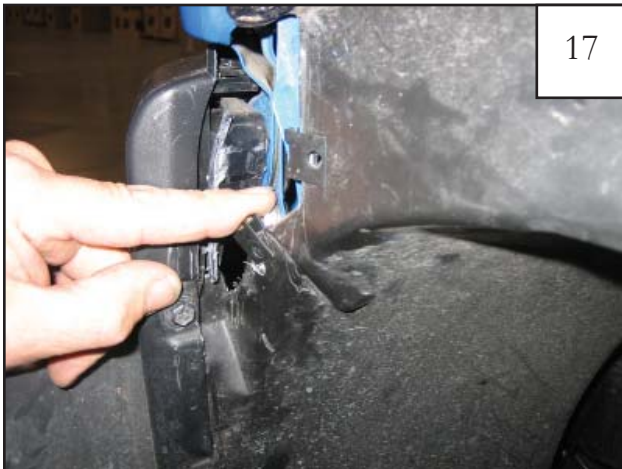
17 Slide supplied Clips (CL1-0022) over holes drilled in previous Step (2 places).
