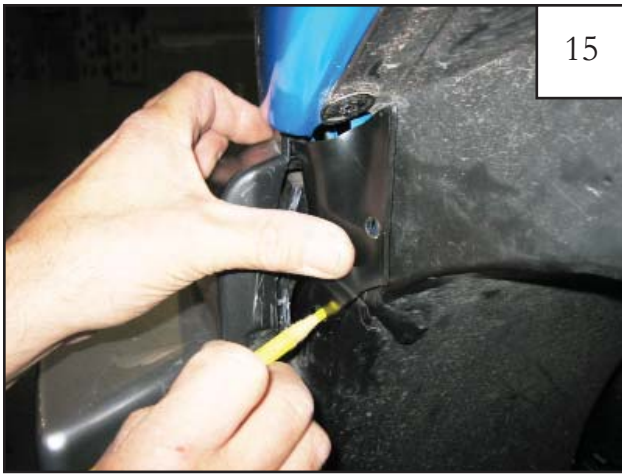
15 Holding Front Inner Piece on front of wheel well next to bumper, use a grease pencil to mark two clip locations.
