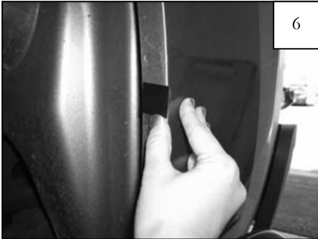
Center a supplied Tab (MT1-0002) over the marks made in step 4, aligning edge of tab with inside edge of fender lip (tab may extend over outside of fender).
