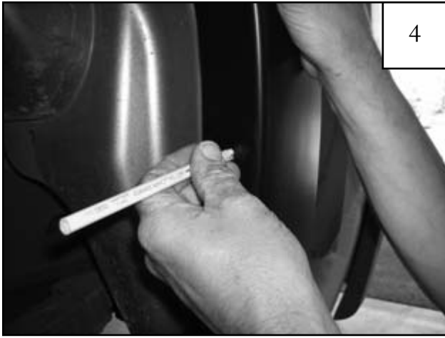
Holding flare in position on fender, use a grease pencil to mark the four clip locations.
