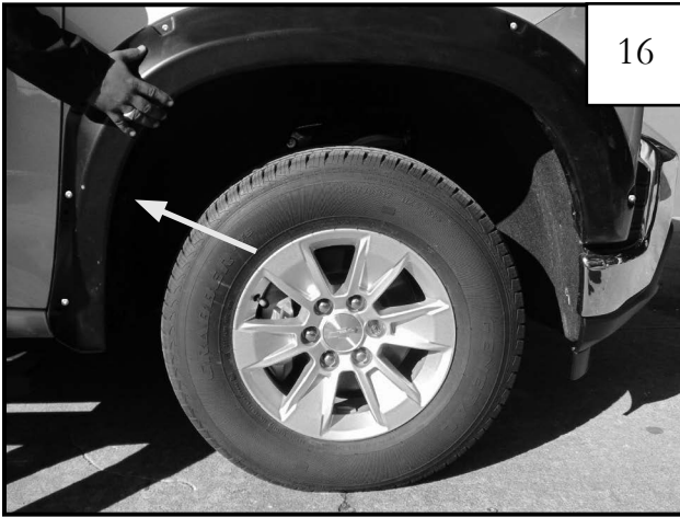
Install (1) supplied phillips head screw (SW1-0058) at rear Clip location. Do not tighten. (If needed use an awl to align flare mounting holes.)
