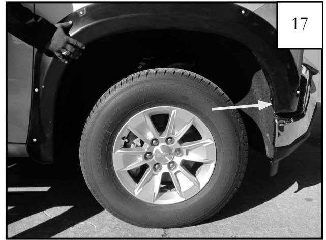
Install (1) supplied phillips head screw (SW1-0049) at front Clip location. Do not tighten. (If needed use an awl to align flare mounting holes.)
