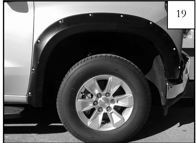
Completed front flare installation.
