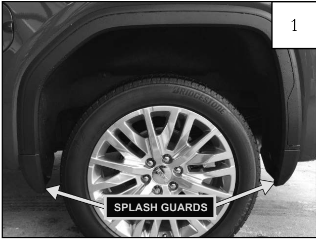
Remove the rear wheel as instructed in your user's manual. Remove the rear splash guards using a T-15 Torx driver.
