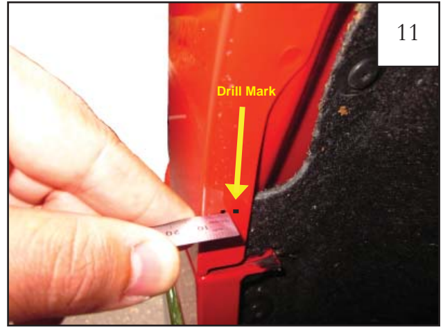
Remove the flare. Using the marks made in step 10 as a guide, measure inward from the outside edge of the fender to verify proper depth of original marked location. Mark must be minimum of 22mm in from outside edge of fender, if short, adjust marks to 22mm.
