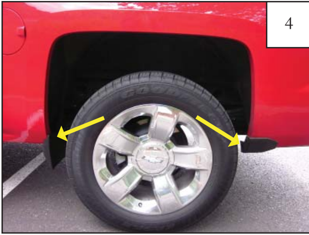
Using a T-15 Torx bit socket wrench, remove factory installed screws. Discard screws.
