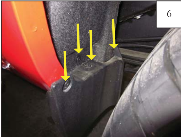
Using a T-15 Torx bit socket wrench, remove the four factory screws from the plastic wheel well piece.
