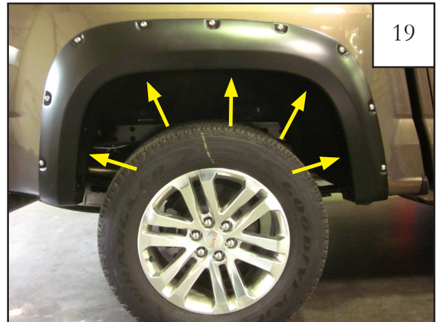
Holding flare in position, use a grease pencil or sharpie to mark the five upper mounting hole locations using the mounting holes in the flare as a guide. Remove flare.
