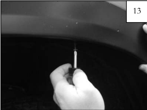
Hold flare to vehicle and start the supplied #8x3/4" Washer Panhead Screws with a Phillips screwdriver. Do not tighten.
