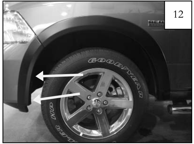
PLASTIC BUMPER ONLY: Additional supplied screw locations.
