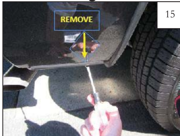
2012 - 2014 Models Only (Optional): Remove inner piece at bottom rear of wheel well using a pry tool.
