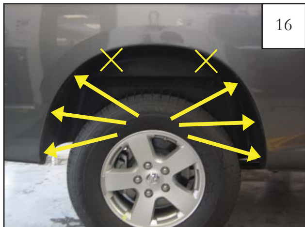
Remove these six factory screws using an 8mm socket wrench. Discard factory screws. X's indicate a factory screw that will not be removed.
