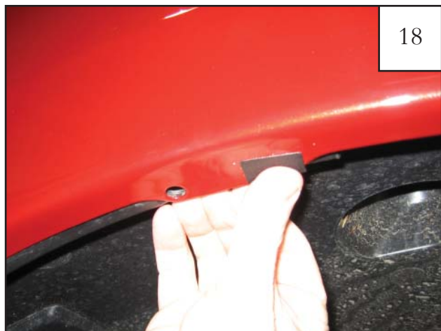
Install Tab (MT1-0014) over existing factory hole.
