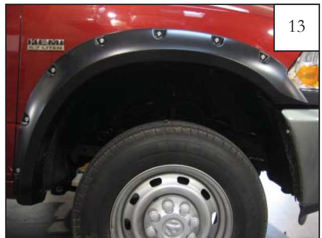
13 Completed front flare installation.
