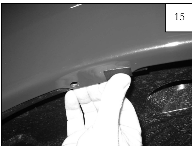
Install plastic tab over existing factory hole.
