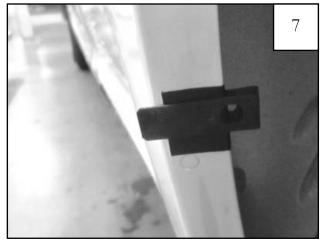
Install a Clip (CL1-0009) over the Tab (MT1-0034) placed in Step 6.
