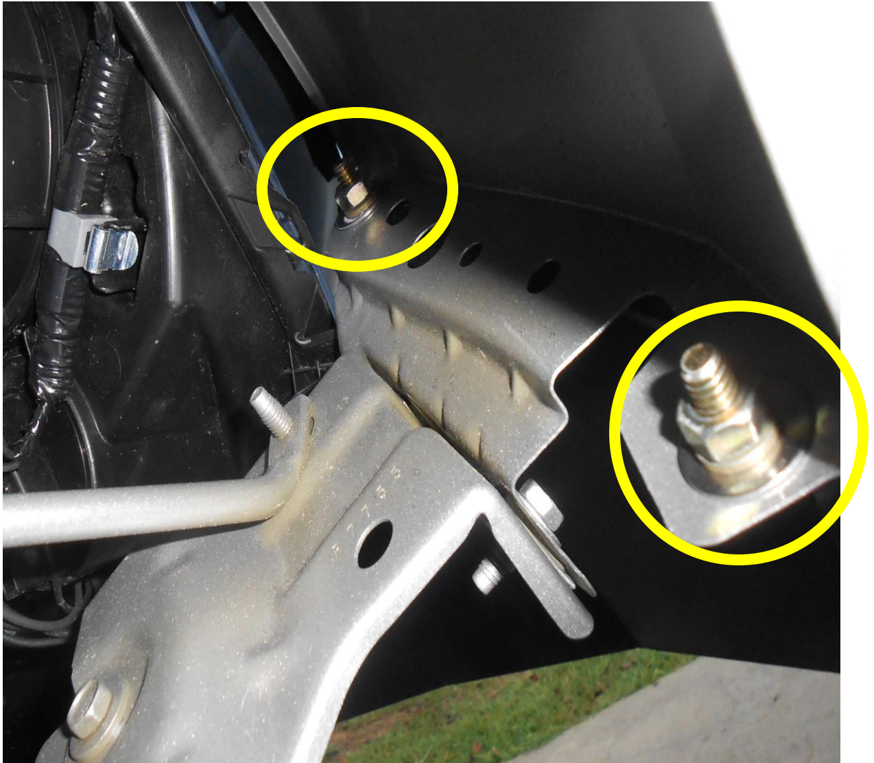
Figure 6b (bolts through mount points on fender)
