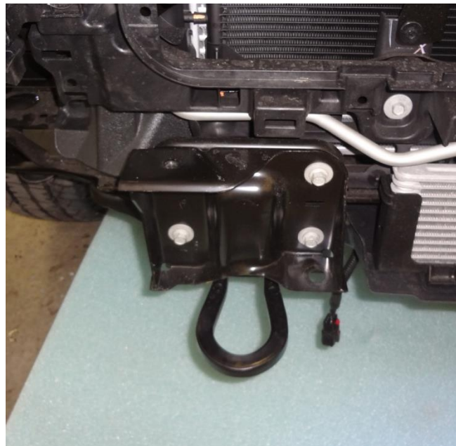
Figure 3b (TOW HOOK & OEM MOUNTING BRACKET)
