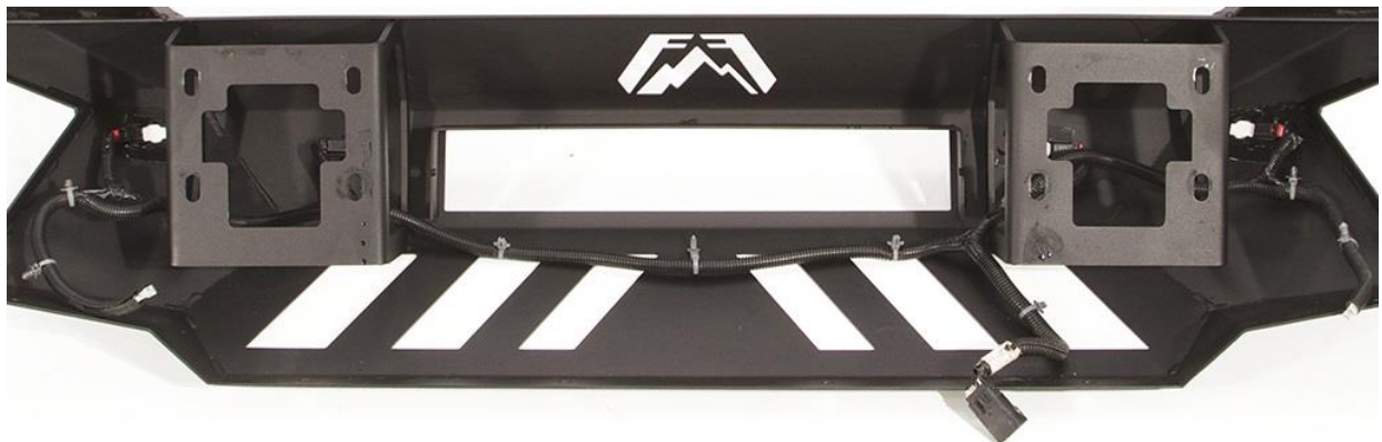
Figure 9a (OVERALL SENSOR HARNESS ROUTING)
