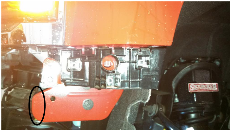
Figure 7a (AREA TO BEND INWARD)
