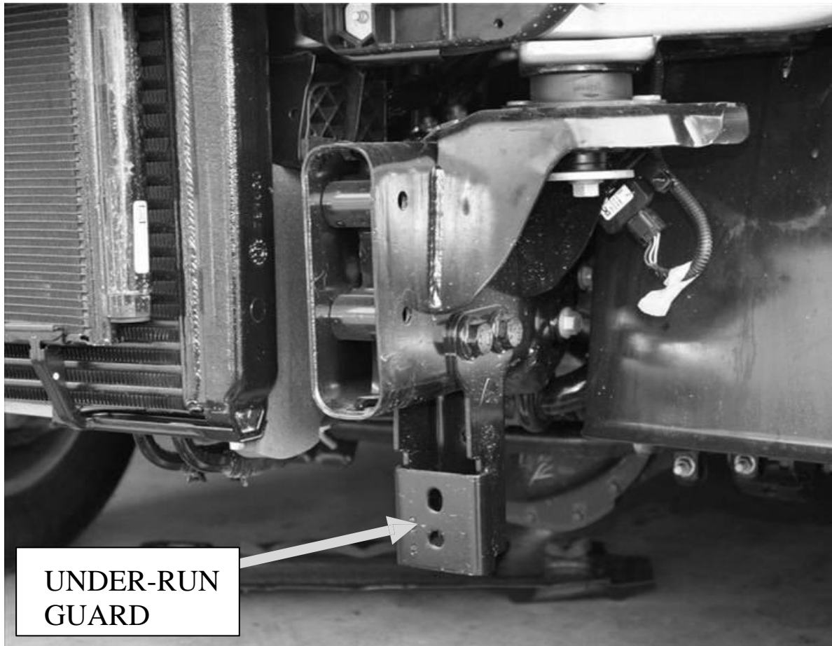
Figure 1 – FRAME UNDER-RUN GUARD (IF EQUIPPED)
