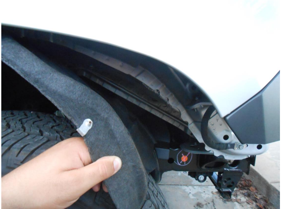
Figure 6a (wheel well liner pull back)
