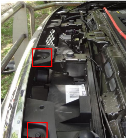
Figure 2a-bolts on LH side
