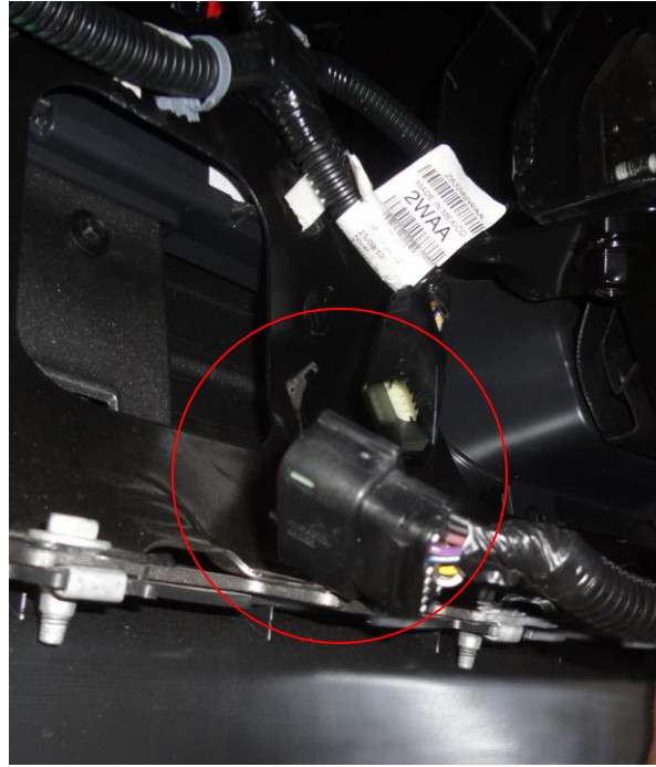
Figure 3(electrical harness disconnected)
