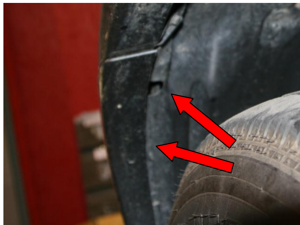
Figure 4 – Fenderwell fastener removal
