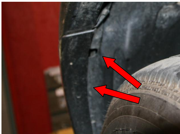
Figure 4 – Fenderwell fastener removal
