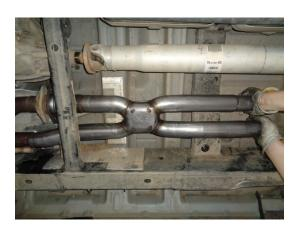
1) Place the new Flowmaster X-Pipe **#26678M** up into position behind the factory front pipes, slide the right side slip connection into the clamp and continue until the flared left connections come together. Using the included 3/8" bolts, nuts and washers, secure the two flanges together. Leave both connections slightly loose for later adjustment if needed.
