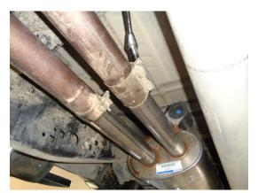
4) Support the muffler with a stand and loosen the clamp on each of the two front inlet pipes using a 15mm socket wrench. Then slide the muffler toward the rear of the vehicle to disconnect the inlet pipes and hangers from the rubber mounts on the vehicle. Lower from the vehicle and set aside.
