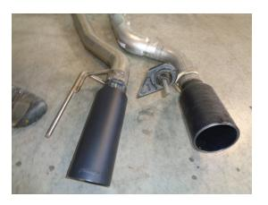
4) Place the new Flowmaster tailpipe assemblies next to the corresponding factory tailpipe. Swap both the front and rear hangers from the factory tailpipes to the new tailpipes.
