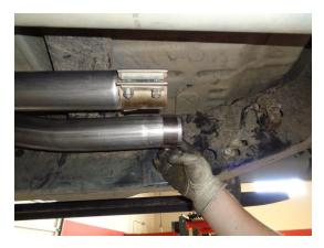
2) Place the factory band clamp from the rear of the resonator onto the left X-Pipe outlet as shown. Place the supplied 2 3/4" clamp onto the right outlet as shown.
