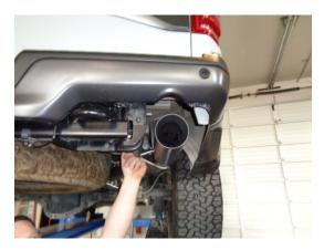
8) Place the ST462B tips onto the end of the tailpipes and adjust to the desired position. Tighten the pinch bolt on the tips enough to hold in position. Check to see that the tip is centered in the bumper cut-out and that there is clearance to the trailer hitch.
