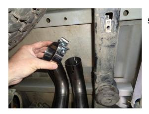
5) Place the provided 3" clamps onto the muffler outlets.
