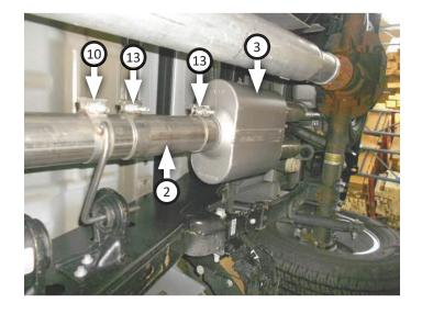
11. Place (x2) clamps (12) onto muffler. Route left front (5) and right tailpipes (4) over axle then connect them to muffler. Insert wire hangers into isolators then tighten clamps just enough to allow for adjustment.
