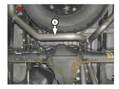
13. Place (x2 ea.) clamps (12) onto side exit pipe (7) then connect them to tailpipes and tighten clamps just enough to allow for later adjustment.
