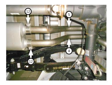
12. Place clamp (12) onto left rear tailpipe (6) then connect it to left front tailpipe. Insert wire hanger into rubber hanger then tighten clamp just enough to allow for later adjustment.
