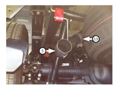
**NOTE:** For a side exit exhaust, complete this step using (x2) **side exit pipes (7)** in place of rear exit pipes.
