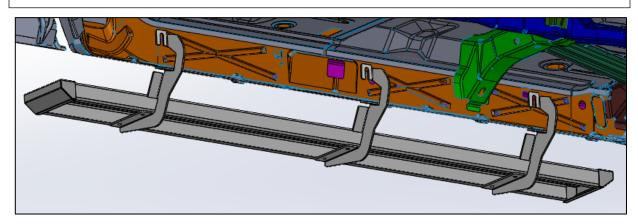
**Step 5:** Insert the supplied threaded brackets (x3) inside the running board lip over the top of each bracket.
