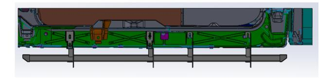
**Step 7:** Insert the supplied threaded brackets (x4) inside the running board lip over the top of each bracket.
