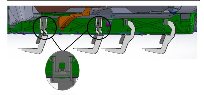
**Step 6:** Set running board along the top of all four brackets and center along the cab.
