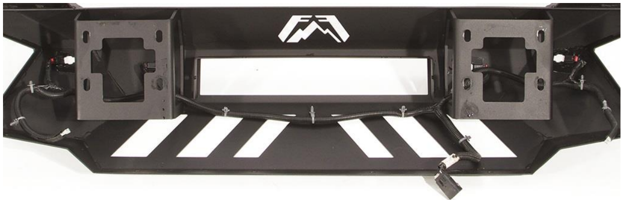
Figure 9a (OVERALL SENSOR HARNESS ROUTING)
