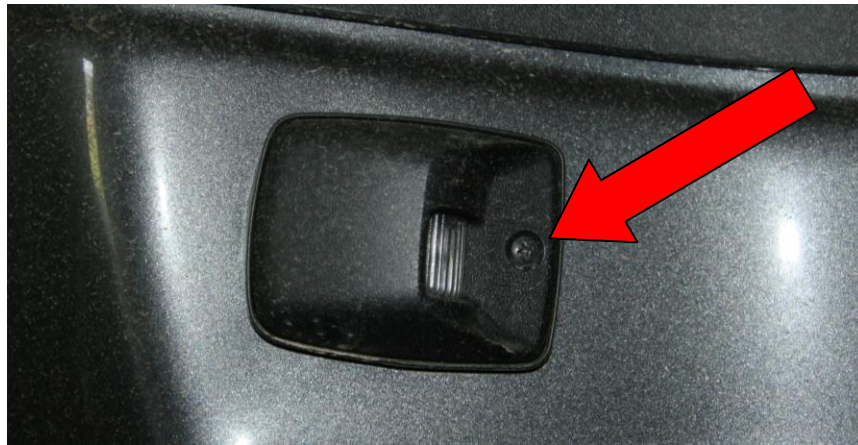
Figure 1 – License plate light removal
