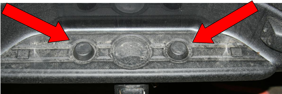
Figure 2 – Bolt cover removal
