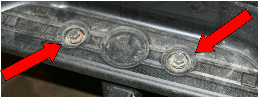
Figure 3 – Trailer hitch bolt removal
