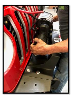
6. If you are going to install our BS10E50W5W, install the light now with the hardware supplied with the light.
