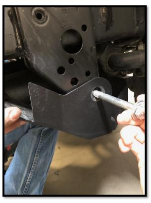
10. Once the two lower skid plate bolts are loosely installed, rotate skid plate up, and use the provided bolts to secure the top portion of the skid plate to the main bumper and wing. Once installed, you can secure the lower frame horn bolts.
