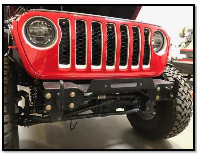
3. Once winch plate is secure, install the main center section of the bumper by sliding it over the top of the winch plate. The bumper should wrap over the D-Ring mounts like shown in image below.
